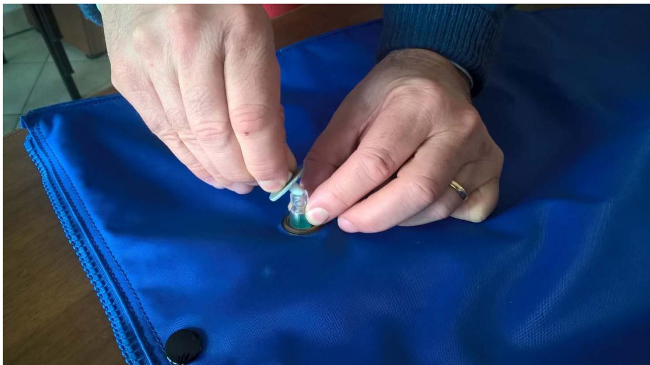
INSERIRE IL NUOVO RACCORDINO (UTILIZZARE UNA GOCCIA DI ATTAK PER FISSARLO STABILMENTE)
